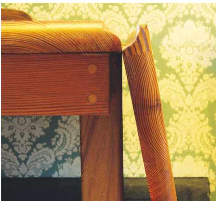
▲ Pic.6 Set the underframe back to avoid this happening!
